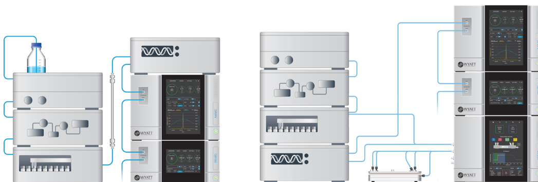
Figure 2: Examples of systems combining size-based separation with in-line light-scattering analysis. Left: an SEC-UV-MALS-dRI system consisting of industry-standard high performance liquid chromatography modules, a DAWN MALS instrument, and an Optilab dRI detector. The size-exclusion column is located between the HPLC system and the detectors. Right: an FFF-UV-MALS-DLS-dRI system, consisting of industry-standard HPLC modules, an Eclipse™ FFF controller and separation channel, a DAWN MALS instrument with embedded DLS module, and an Optilab dRI detector. Credit: Wyatt Technology
